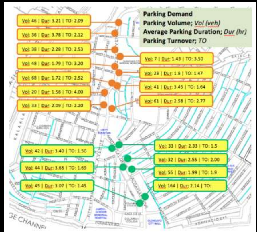
Parking Volume, Parking Duration, and Parking Turnover along Rizal Avenue North Side
