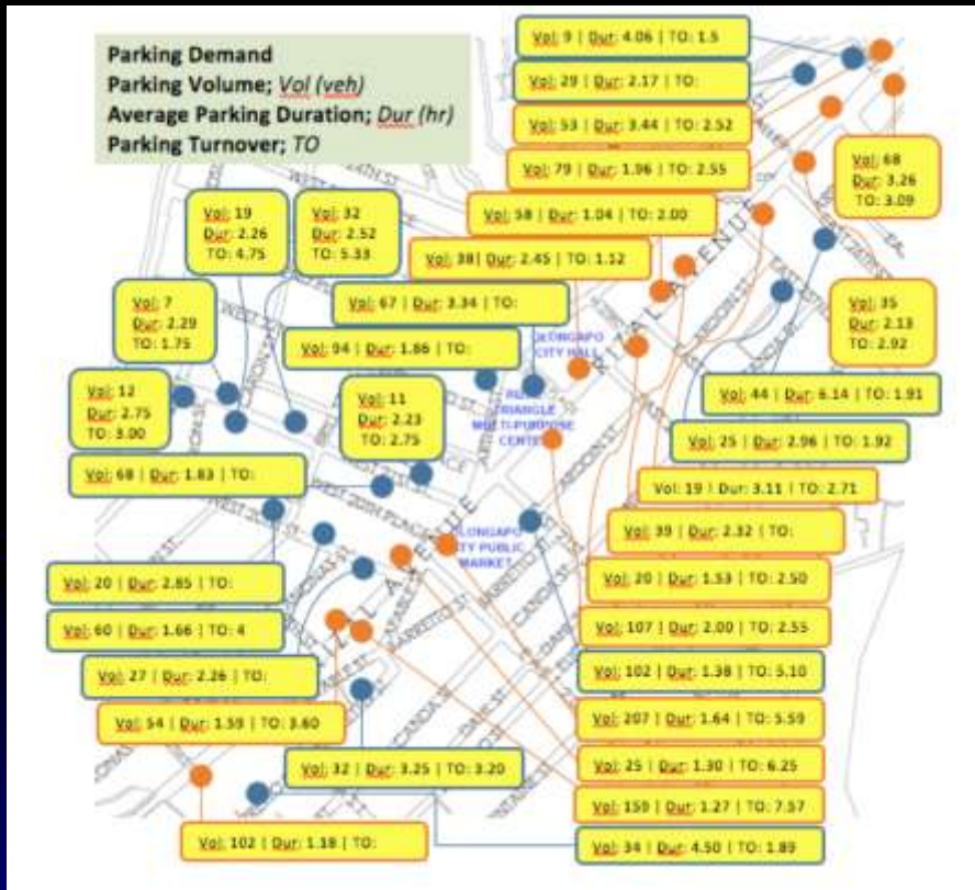
Parking Volume, Parking Duration, and Parking Turnover along Rizal Avenue South Side
